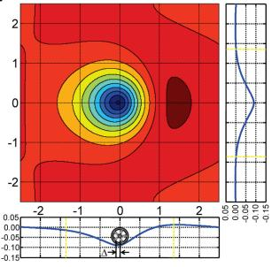
The figure shows a sample output of the model: a contour plot of pavement deflection and deflection in two perpendicular directions.
