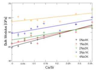
Fig. 1: Bulk modulus (a measure of stiffness) of the glass vs. Ca/Si ratio with various Na-K repartitions.
