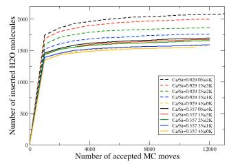
Fig. 2: Water uptake for low Ca/Si ratio (dotted lines) and high Ca/Si ratio, with various Na-K repartitions as a function of the number of accepted Grand Canonical Monte Carlo (GCMC) moves.
