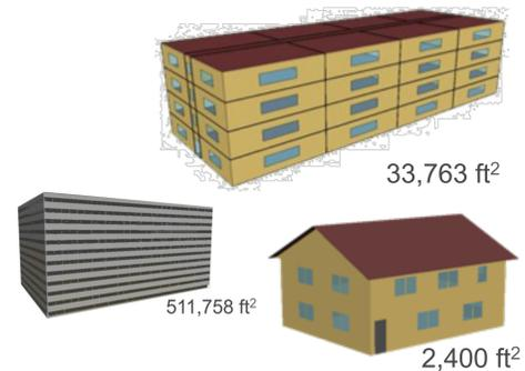
Two code-compliant designs were analyzed in each building category; wood and concrete two-story single-family homes (2,400 sf), wood and concrete four-story multifamily (34,000 sf), steel and concrete 12-story commercial (500,000 sf) buildings.
