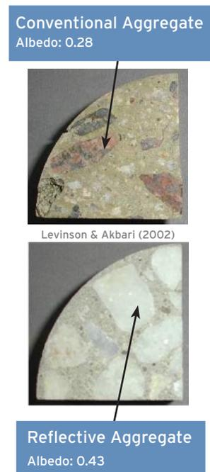
**Figure 2.** A comparison between conventional and reflective paving strategies. Changes to the binders, aggregates, or surface properties of a pavement can substantially increase its albedo.
