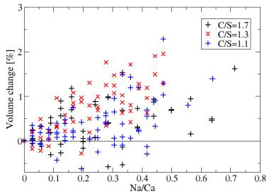
Fig. 1: Simulated C-S-H volume change as a function of the sodium to calcium ratio, for three initial C-S-H compositions at 0K.
