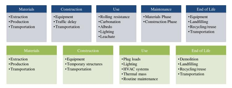
Figures 1 and 2: Typical phases and components of the pavement (top) and building (bottom) life cycles
