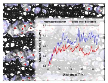
Molecular scale representation of the water trapped in C-S-H gel nanopores. The Ca-O-Si layers are depicted in black, molecular water molecules in white and red, and the pore space in blue. The insert shows the increase in the maximum shear stress after molecular water dissociation to OH<sup>-</sup>.
