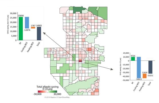
**Figure 7.** GHG savings from building energy demand (BED) and radiative forcing (RF) over 50 years in Phoenix, AZ due to a 0.2 increase in pavement albedo by using portland cement concrete instead of asphalt. 'Cooling BED' refers to cooling usage, while 'Heating BED' refers to heating usage. Negative values indicate a GHG burden.
