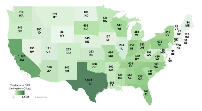
Figure 3. The annual global warming potential savings due to increasing the surface reflectivity of all pavements across the continental U.S.
