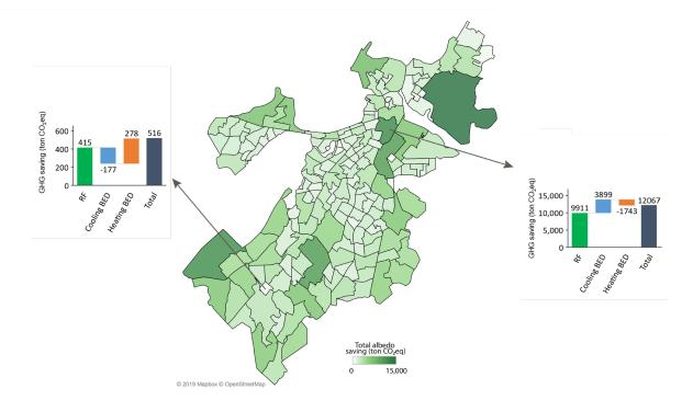
**Figure 6.** GHG savings from building energy demand (BED) and radiative forcing (RF) over 50 years in Boston, MA due to a 0.2 increase in pavement albedo by using portland cement concrete instead of asphalt. 'Cooling BED' refers to cooling usage, while 'Heating BED' refers to heating usage. Negative values indicate a GHG burden.
