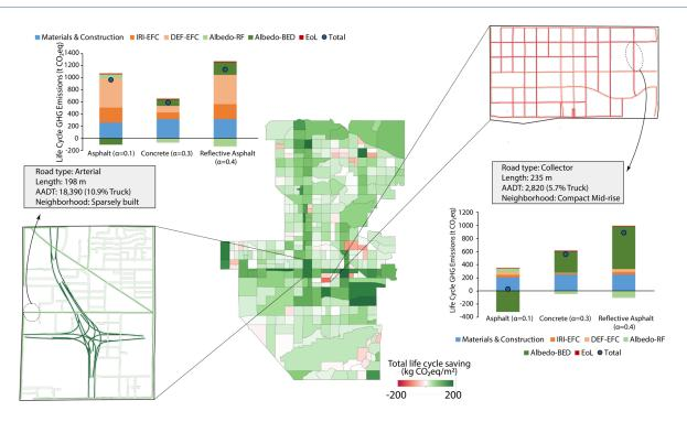
**Figure 8.** Life cycle GHG savings of replacing asphalt concrete with portland cement concrete in Phoenix, AZ. The bar charts compare life cycle GHG emissions of two cool pavement strategies to the currently built asphalt for the specified road segment.
