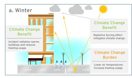
Figure 4. The climate change impacts of reflective pavements in cities during winter (a) and summer (b). While reflective pavements always reduce air temperatures and exert radiative forcing benefits, their impacts on building energy demand oscillate seasonally due to changes in HVAC demands and air temperatures.
