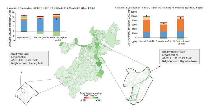
**Figure 9.** Life cycle GHG savings of replacing asphalt concrete with portland cement concrete in Boston, MA. The bar charts compare life cycle GHG emissions of two cool pavement strategies to the currently built asphalt for the specified road segment.
