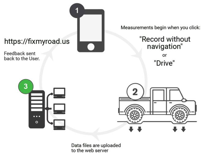
‘pulses.’ Carbin then uses CSHub research to convert these ‘pulses’ into the international roughness index, which is the standard for measuring pavement roughness.
