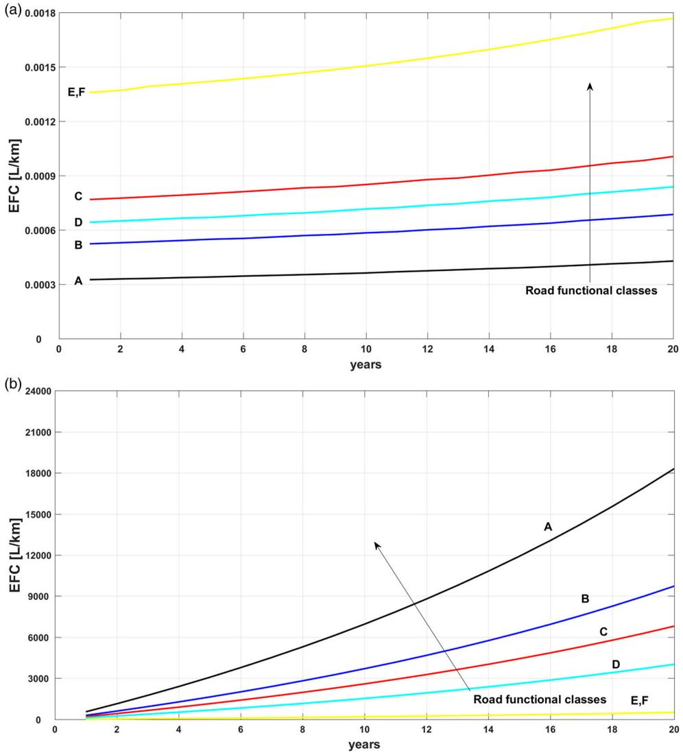
Figure 13. Difference in deflection-induced EFC over time including pavement deterioration compared to the case of constant stiffness for all of the road classes defined in Table 2 (a) for a single ESAL, and (b) including traffic volumes.
