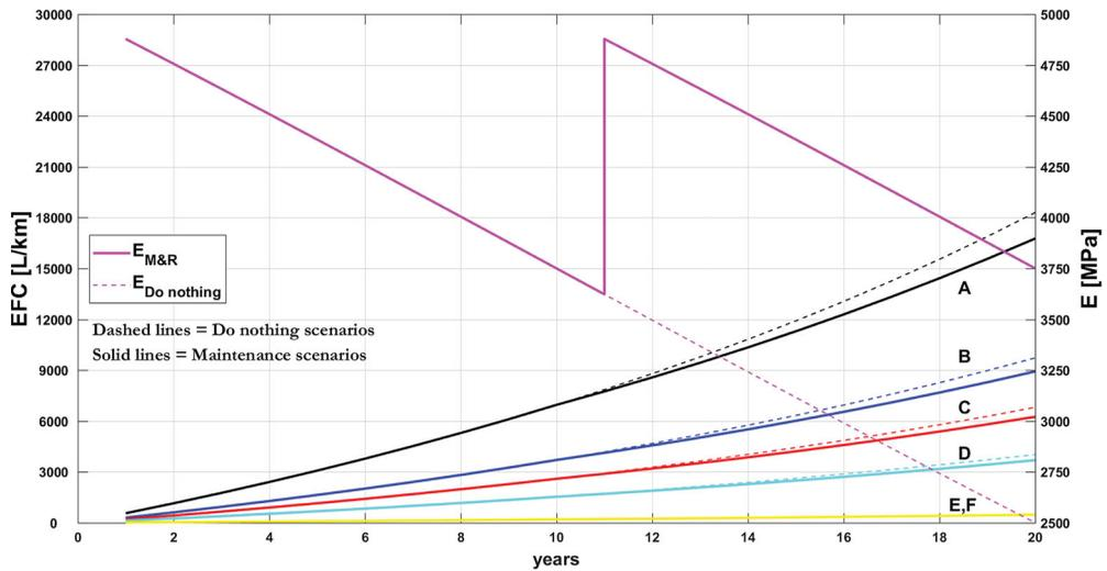
Figure 14. Difference in deflection-induced EFC over time including pavement deterioration compared to the case of constant stiffness for all of the road classes defined in Table 2 and full traffic volumes for do-nothing (solid lines) and maintenance (dashed lines) cases. Stiffness over time is plotted on the right axis.
