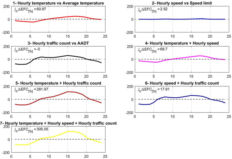
Figure 11. Percent difference in deflection-induced EFC as a function of time of day for an asphalt pavement segment compared to baseline calculations made using average and constant values for the scenarios outlined in Table 3. Each plot lists a cumulative daily EFC percent difference,  $\int \Delta EFC$ , which accounts for positive and negative differences.
