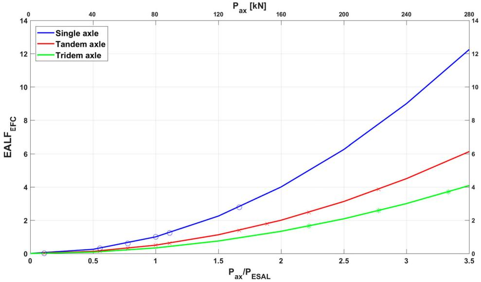
Figure 4. Conversion factors of deflection-induced EFC caused by different axial loads.
