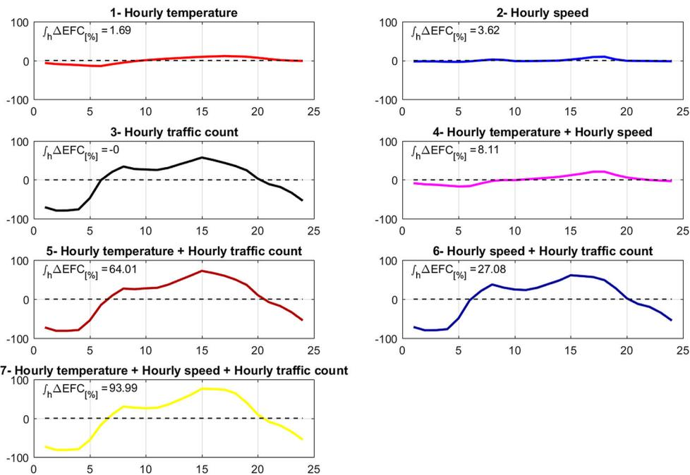
Figure 12. Percent difference in deflection-induced EFC as a function of time of day for a concrete pavement segment compared to baseline calculations made using average and constant values for the scenarios outlined in Table 3. Each plot lists a cumulative daily EFC percent difference,  $\int \Delta EFC$ , which accounts for positive and negative differences.
