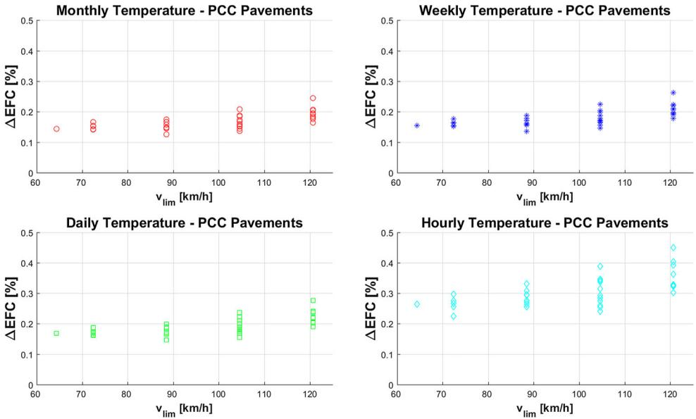
Figure 6. Percent increase in EFC of concrete pavements due to deflection-induced PVI using hourly, daily, weekly, and monthly temperatures, compared to annual temperatures.
