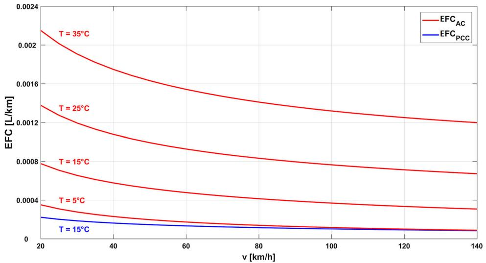
Figure 7. EFC due to deflection-induced PVI as a function of vehicle speed at a range of constant temperatures for both asphalt (AC) and concrete (PCC) pavements.
