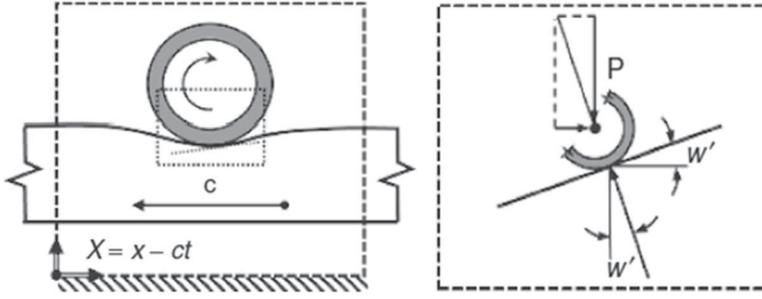
Figure 1. (a) Pavement-vehicle interaction in moving coordinate system. (b) Magnified detail of the slope under the wheel (from Louhghalam et al. 2014a).
