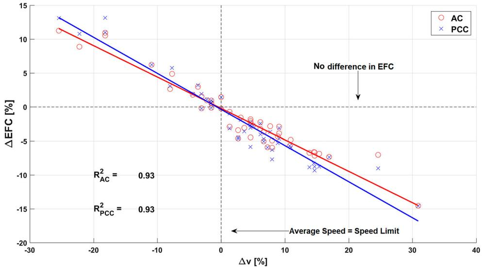
Figure 8. Percent difference in EFC due to deflection-induced PVI for annual average hourly-recorded speed compared to the baseline speed assumption of the speed limit for Arizona pavement segments. The x-axis is the percent difference in annual average hourly-recorded speed compared to the speed limit. Lines are fits for the asphalt data points (red) and concrete data points (blue), with the goodness of fit parameters shown on the plot (colour online only).
