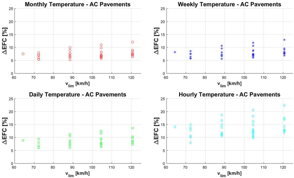
Figure 5. Percent increase in EFC of asphalt pavements due to deflection-induced PVI using hourly, daily, weekly, and monthly temperatures, compared to annual temperatures.
