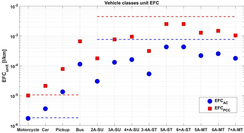
Figure 2. EFC values for higher resolution data for axial load configuration (FHWA classifications listed on  $x$ -axis and blue circles for PCC and red squares for AC) and for simplified classifications (blue dashed lines for PCC and red dashed lines for AC) (colour online only).
