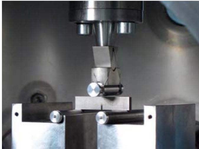
*Figure 3: A traditional fracture toughness test mechanism*
