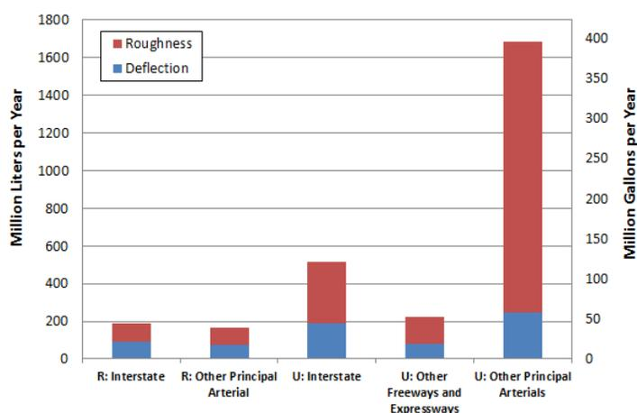
Excess fuel consumption per year on rural (R) and urban (U) highways, due to pavement deflection and roughness at 95% confidence interval. Pavement properties, roughness, and traffic volume have been extracted from the LTPP database and the FHWA Highway Statistics manual.
