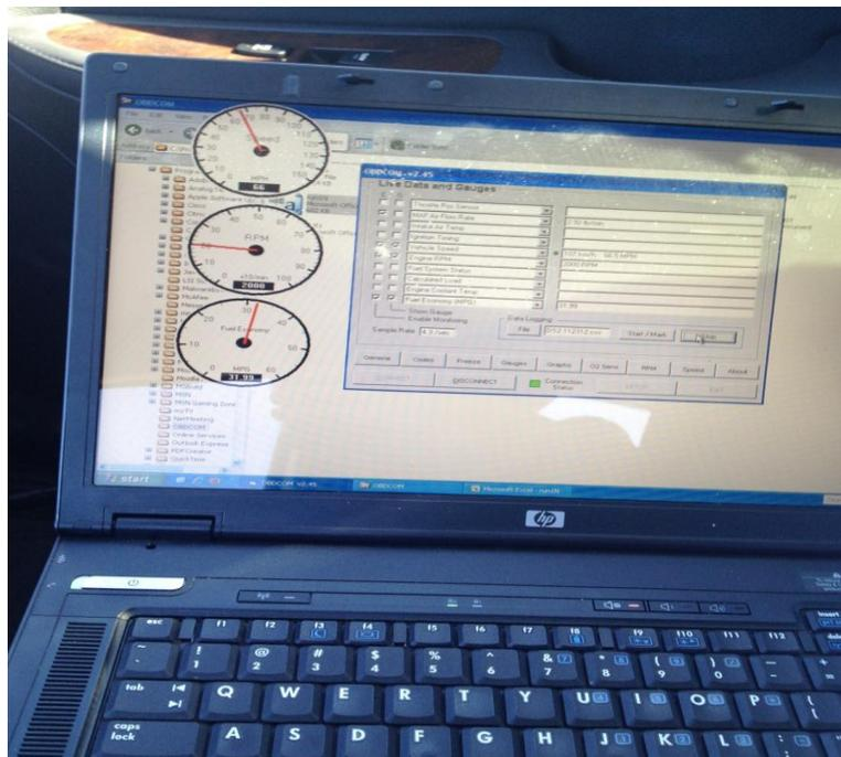
**Figure 6. Real-time Data Collection of Real-Time Fuel Consumption and Vehicle Speed.**
