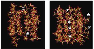
Connectivity among silica tetrahedra in C-S-H at different water content levels, where yellow chains are silicates. At molar ratio  $H_2O/Si = 0.967$  or ~80%RH, only two points of connection exist between the two silicate-rich layers of a C-S-H unit cell (at #), However, at  $H_2O/Si = 0.017$  or i1%RH, three times more connections exist (at \*).
