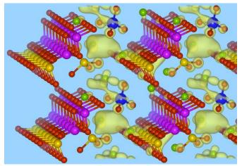
Localized electron clouds (light yellow) in an aluminum and sulfate doped belite crystal obtained by quantum simulations. Green, orange, red, blue, pink spheres represent Ca, Si, O, S, and Al atoms, respectively.
