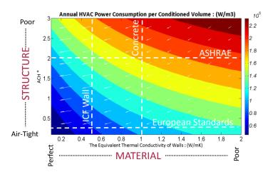
Sample output: Isovalue map of annual HVAC power consumption in function of air tightness (ACH\*=Air Change per Hour under atmospheric pressure differential) and material performance (thermal conductivity) for a residential home unit in Boston, MA. ACH=2.0 is an upper ASHRAE-reported value. The arrays indicate the highest slope for residential energy savings.
