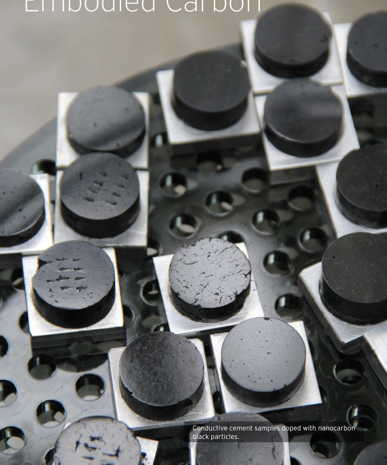
Conductive cement samples doped with nanocarbon black particles.
