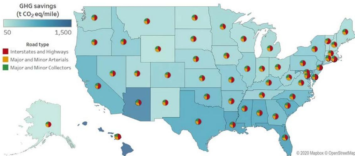
The map above shows the potential reductions in overall greenhouse gas emissions from the transportation sector as a consequence of stiffening pavements nationwide. The data derives from research that appeared in the *Transportation Research Record*.
