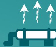
**2.** You also need cement, which is made at high temperatures in a kiln. The process releases CO<sub>2</sub>, which can be captured to replace the need for CO<sub>2</sub> from another industrial source.
