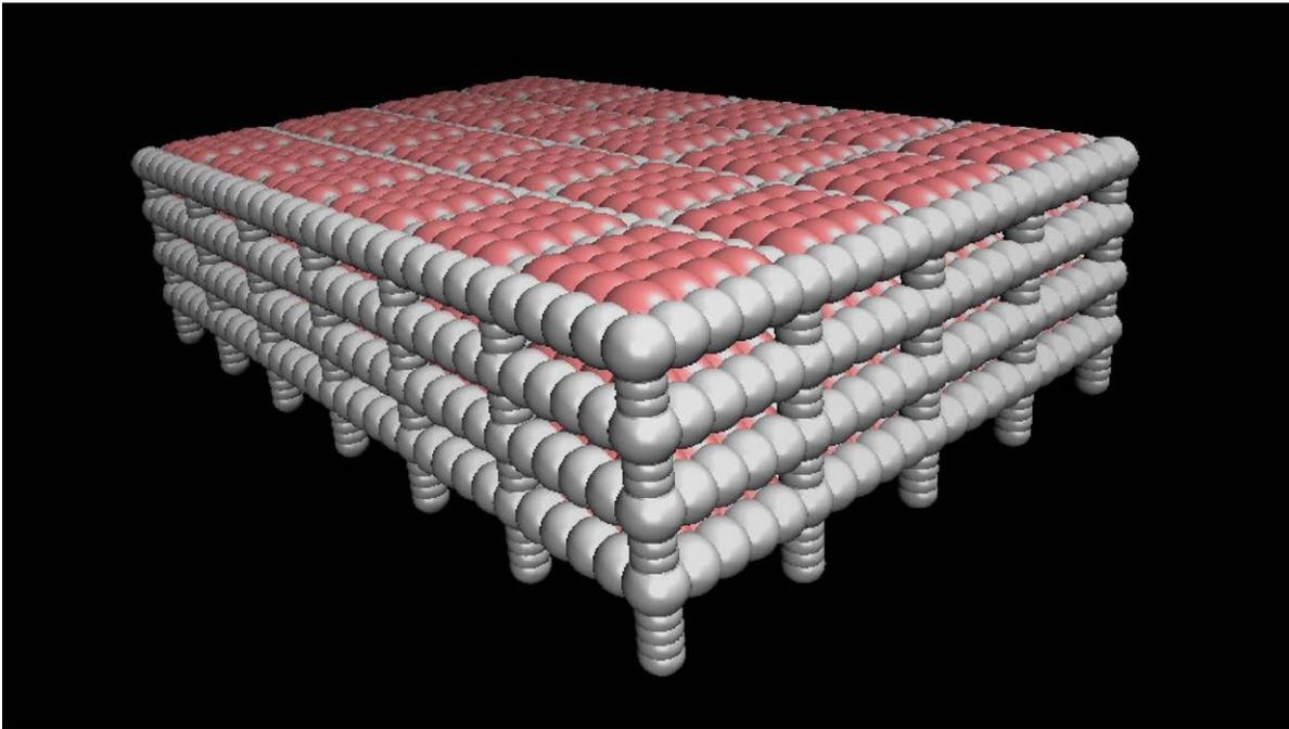
Inspired by molecular dynamics, CSHub research assistant Kostas Keremidis models buildings as an ensemble of atoms. Though unconventional, such an approach has allowed him to predict building failure far more quickly than with traditional methods such as Finite Elements.
