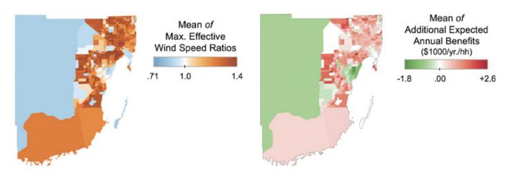
By applying CSHub's city texture modeling approach, research assistant Bensu Manav has identified gaps in conventional loss estimation tools. The figures above show how modeling urban layouts captures wind load amplifications (wind speed ratios) and potential annual savings if city texture informed mitigation.
