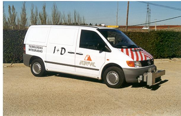
**Figure 1. An example of a vehicle fitted with roughness measurement equipment (Photo credit: Grupo Inzamac)**
