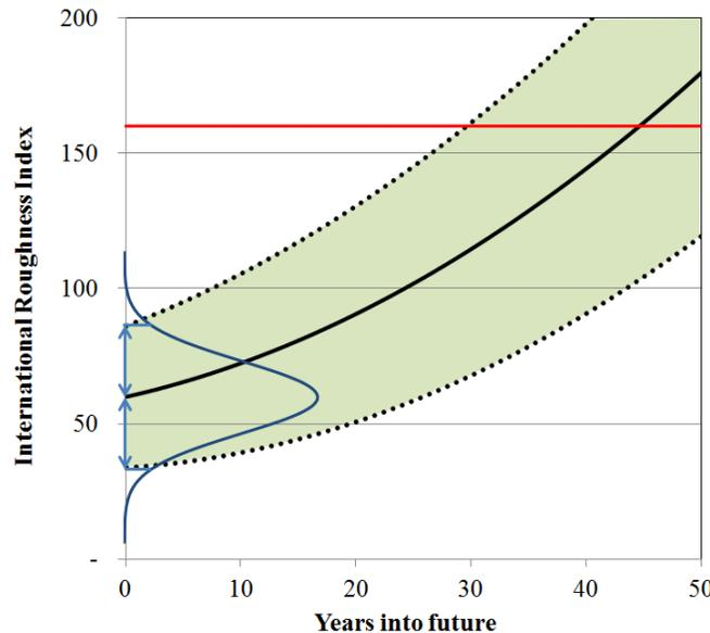
Figure 1 – Sample MEPDG prediction of the evolution of IRI for a pavement alternative at a reliability of 90% (top dashed line) 50% (solid line) and 10% (bottom dashed line)
