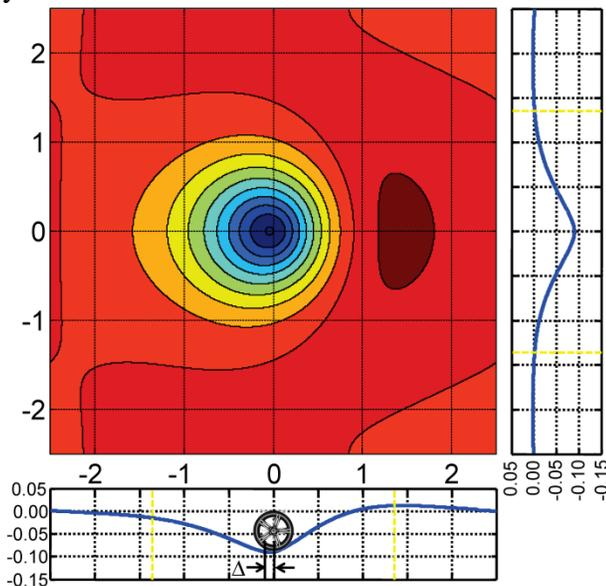
The figure shows a sample output of the model: a contour plot of pavement deflection and deflection in two perpendicular directions.
