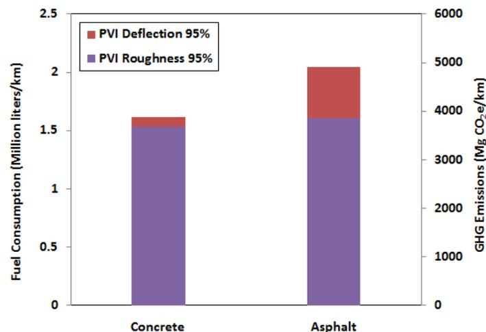
Sample Output: Excess fuel consumption and resulting CO<sub>2</sub>e emissions for two high-volume pavement systems for a 50 year design life using a 95% confidence interval. (Two-lane kilometer section design from Athena (2006); AADT=15,000; AADTT 1,500; AC maintenance at years: 17, 28, 38, 47; PCC maintenance at years 20, 40).
