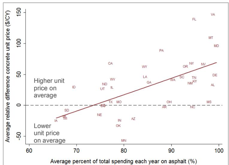
Comparison between the average relative difference unit price of concrete and the 2005-2014 average percent of total spending on asphalt in the 44 states with concrete spending. Zero is the average unit price across all states, and higher average relative difference unit price indicates a higher unit price for a state.
