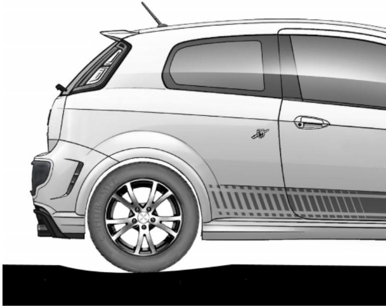
When the tires of a car or truck roll over a roadway, the maximum pavement deflection is just behind the path of travel. This has the effect of making the vehicle's tires roll continuously up a slight slope (exaggerated in this illustration), increasing the vehicle's fuel consumption.
