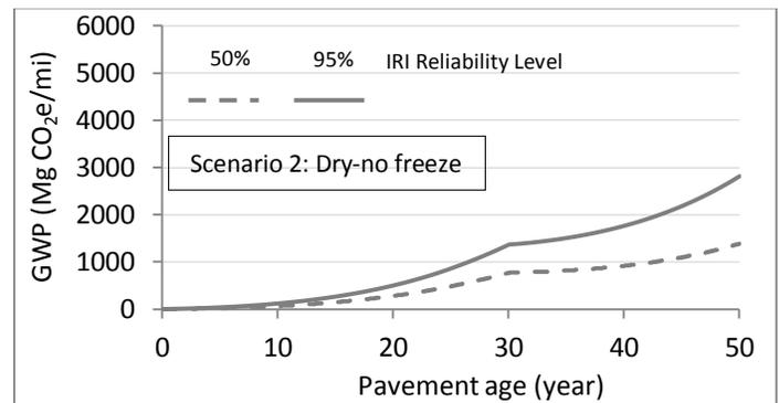
Figure 1: Progression of IRI-induced global warming potential over pavement age based on 50% and 95% levels of reliability.
