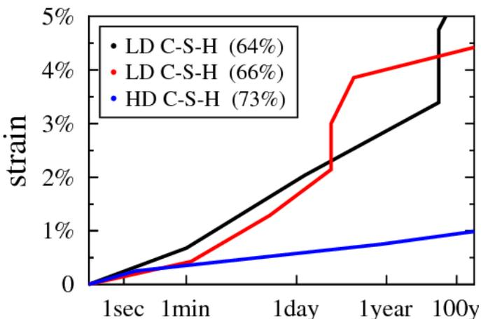
Creep curves for low-density (LD) C-S-H gels (solid fractions 64% and 66%) and high-density (HD) C-S-H gels (solid fraction 73%). The applied shear stress is 100 MPa for the LD C-S-H systems, and 280 MPa for the HD one (70% of the failure stress in both cases). The horizontal axis of time is in logarithmic scale. The linear trends of the strain in this scale indicate logarithmic creep. Note that the HD gel creeps much less than the LD ones.
