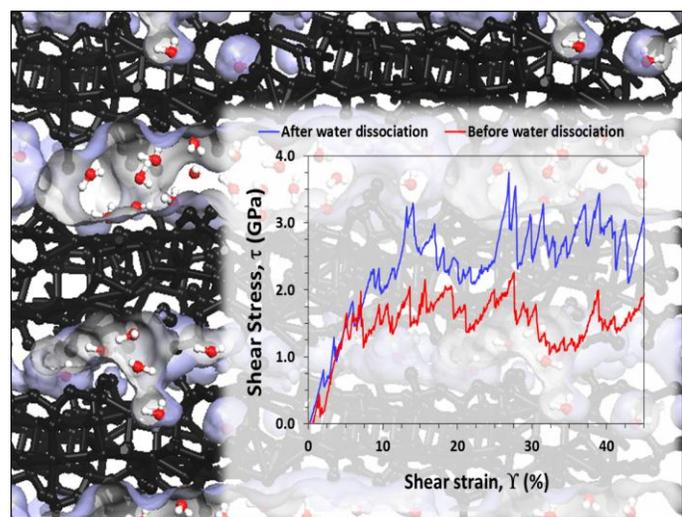
Molecular scale representation of the water trapped in C-S-H gel nanopores. The Ca-O-Si layers are depicted in black, molecular water molecules in white and red, and the pore space in blue. The insert shows the increase in the maximum shear stress after molecular water dissociation to  $OH^-$ .
