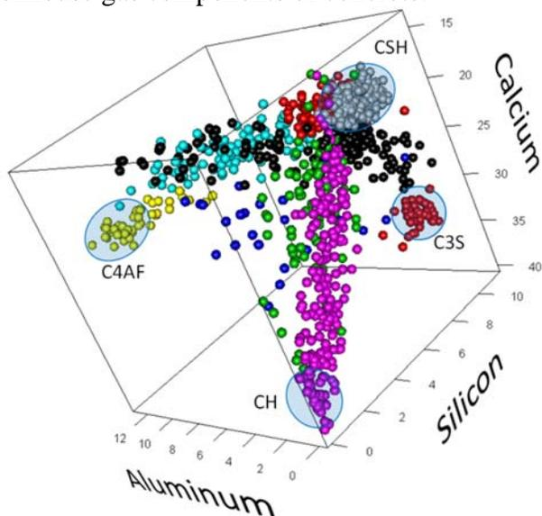
*In situ* assessment of cement chemistry by statistical cluster analysis of wavelength dispersive spectra for a specific Portland cement (OPC). Colors represent different phases in hardened cement paste as identified by this analysis. Units in atomic percent (number of atoms/total number; except H).
